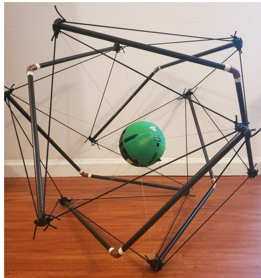
Figure 9: Flounder 3.1 - 6 Motors, Integrated Microcontroller
