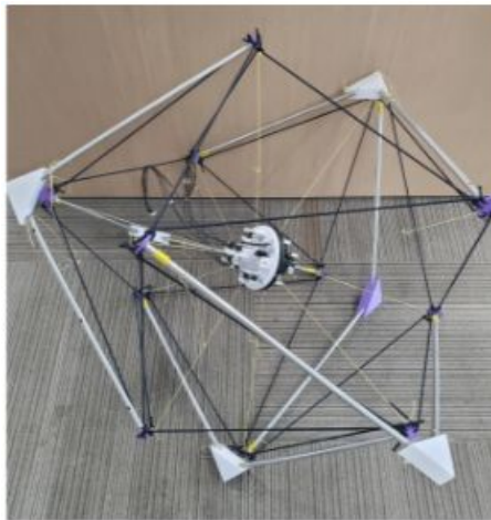
Figure 2: Flounder 1.0 - 12 Motors and Original Bent Rods
