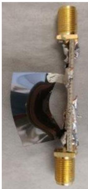
Figure 22. MXene capacitors with copper leads attached.
