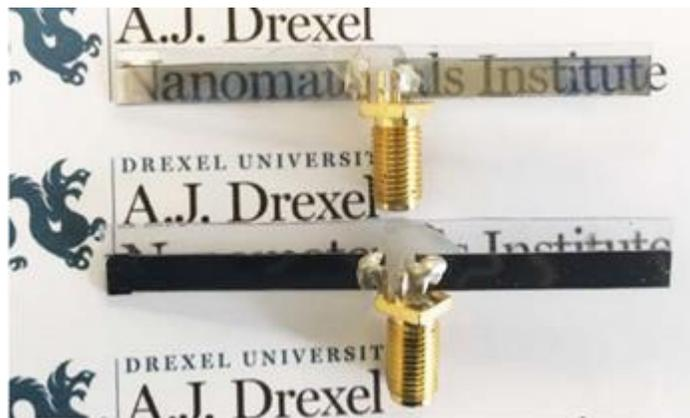
Figure 2. Transparent MXene Dipole Antennas of a) 62-nm-thick and b) 1.4- $\mu\text{m}$ -thick [10]
