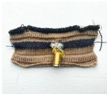
Figure 5: Knitted antenna using MXene-coated nylon yarns as the conductive material and uncoated yarns for the non-conductive material. SMA connectors were sawed and connected to MXene-coated yarns using conductive epoxy.
