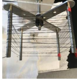
Figure 10. Nylon with 30 coats of MXene colloid on yarn coater's winder.
